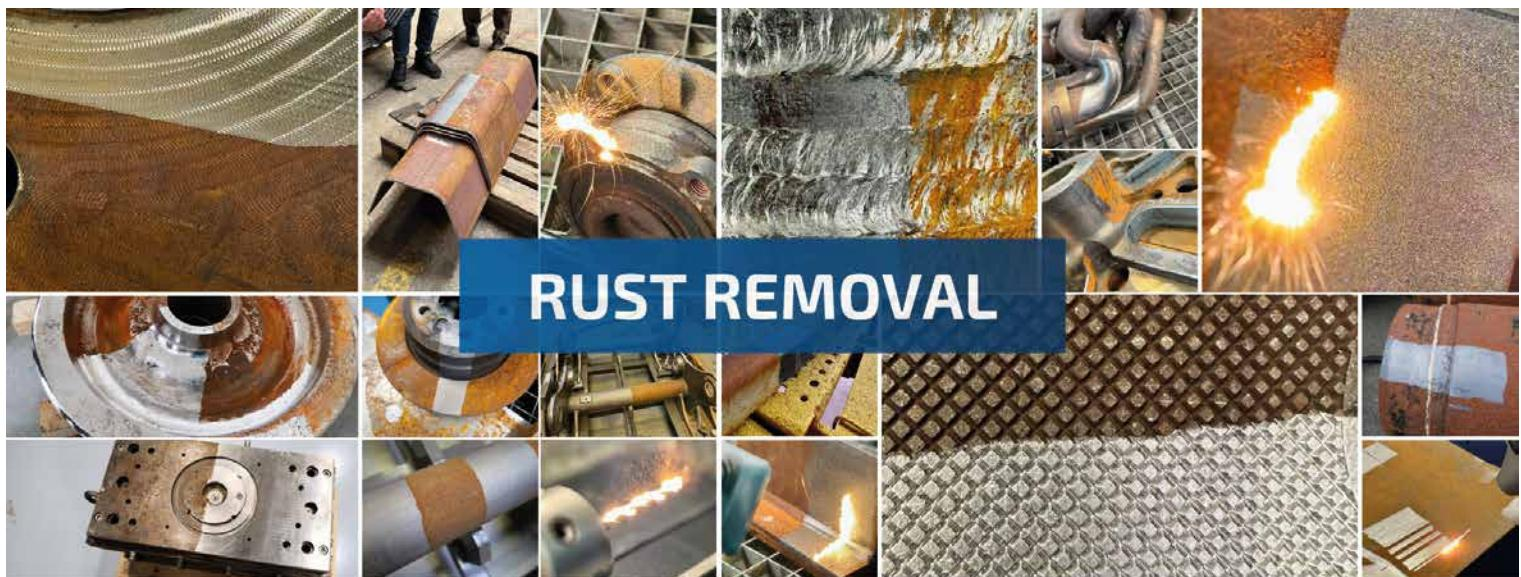
**Rust removal:** cleaning lasers are ideal for removing rust from steel structures, machine parts, tools, pipes and vehicles. This method is fast, does not damage the underlying material and eliminates the need for abrasive or chemical processes.
