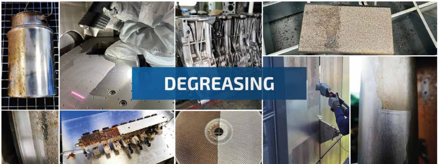
**Degreasing:** lasers are often used to remove oil, grease and other oily contaminants from the surfaces of automotive parts, machine components and tools. This prepares parts for further processing such as welding, painting or bonding.
