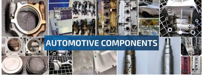
Automotive components: laser cleaning is widely used in the automotive industry to remove dirt, adhesive residues, lubricants or oxides from components. It is used, for example, in brake discs, engine parts, or in the preparation of surfaces for bonding and painting.
