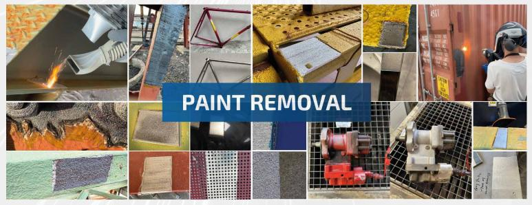
**Paint removal:** lasers gently and precisely remove paint and varnish from metals and other materials, ideal for the aerospace, automotive or antique restoration industries
