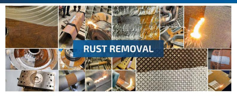
**Rust removal:** cleaning lasers are ideal for removing rust from steel structures, machine parts, tools, pipes and vehicles. This method is fast, does not damage the underlying material and eliminates the need for abrasive or chemical processes.
