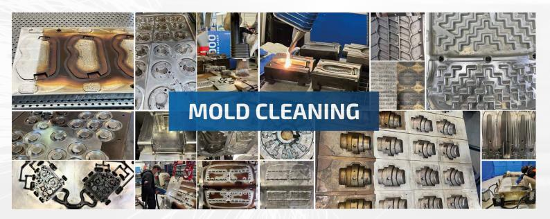
**Mold cleaning:** in the plastics, rubber and metalworking industries, lasers are popular for cleaning molds of deposits and material residues without disassembly. This minimizes downtime and increases production efficiency.
