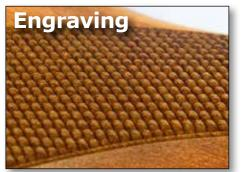
Stable operation over a wide range of settings enables precise control of material removal, allowing consistent ablation depth or detailed 3D engraving.
